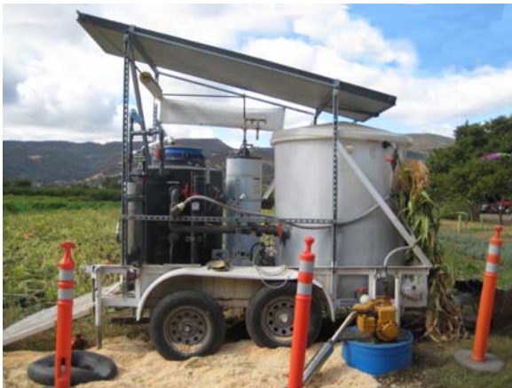
Prototype standalone trailer-mounted steady system with solar thermal collector by Sustech
